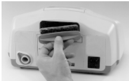
Figure 7. Removal of Filter Drawer
