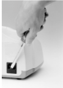
Figure 8. Removal of Fuse Holder
