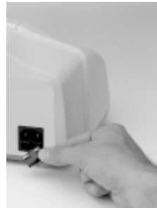
Figure 9. Replacement of Fuse
