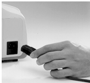
Figure 3. Power Cord Connection to Inlet
